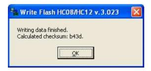
Now the new firmware (update) is installed on the PLC. Click "OK" button and disconnect the interface from PC to PLC.
