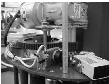
Figure 8: Option kit 16.8242 mounted properly?
