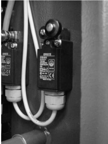
Figure 4: Are the limited switches of the filmcarrige working correctly
