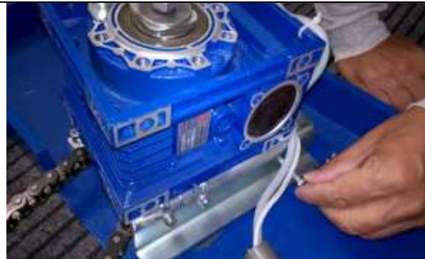
Fig.5 Insert N°1 M6 long screws (left side) to hold the rectangular plate
