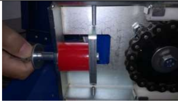
Fig.9 Put the group (big bolt - red polizene – rectangular plate) online with 2 M6 long bolts
