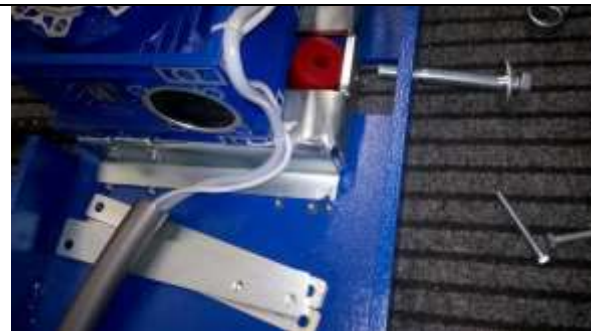
Fig.2 Unscrew the bolts that fix 3 plates (opposite side of the motor)
