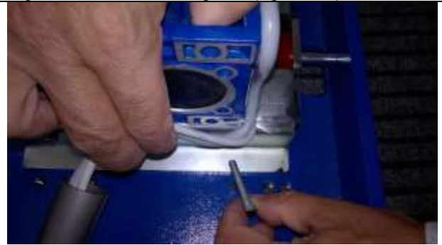
Fig.16 Unscrew M6 long bolt (left side)
