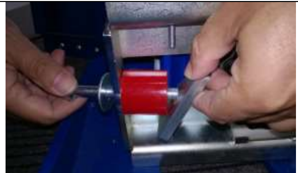
Fig.8 Screw to the rectangular plate
