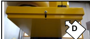
D = Anti-crushing device
