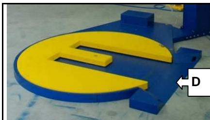
D = Anti-crushing device
