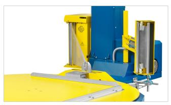
Incorporating all belonging functions of attaching, clamping, cutting and wiping the film end to the package.
