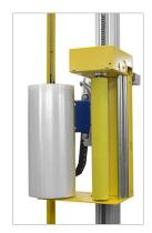
In addition, with larger volumes, different sizes and types of products, the user has a choice of the **CA6** carriage with a **1 motor powered film roll brake** (fixed pre-stretch of 150, 200 or 250%) or the **CA7** carriage with two motor-driven **power pre-stretch**. Delivering between 120 and 350%. (1 meter becomes 4,5 meters of film).
